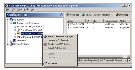
Figure 3-1. Right-Click a VXI System in MAX to Run Resman on that System
